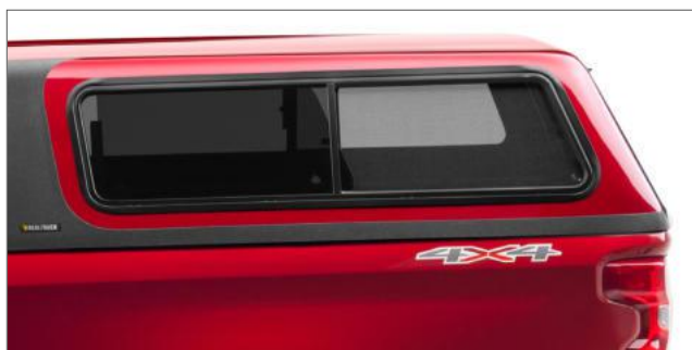
Aluminum-framed sliding side window with screen
