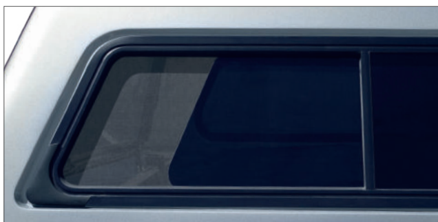
Recessed side sliding window with screens and corner fascia
