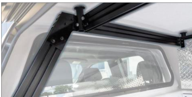
Patented internal aluminum skeleton
