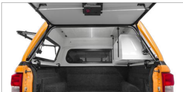
Toolboxes securely fastened to roof framework
