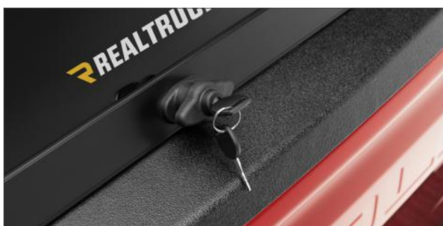
Composite single T-handle with factory-grade lock cylinder
